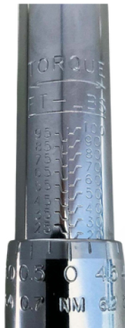
Figure 4. Torque wrench showing adjustment range of 20-100 ft. lbs.
