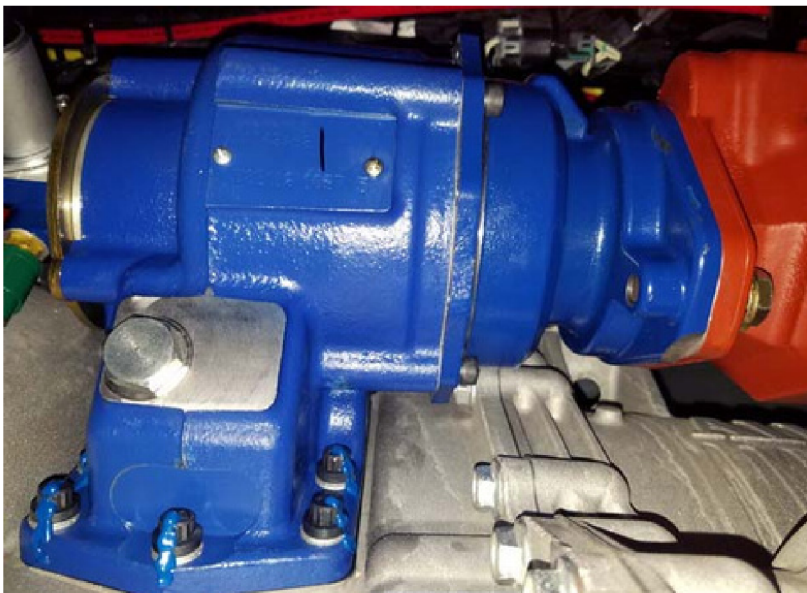
Figure 7. PTO installation with witness marks painted onto torqued capscrews.
